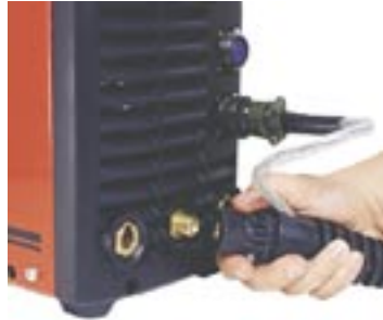
Installing gas-cooled torch
