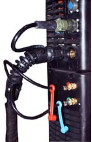
Installing water-cooled torch
